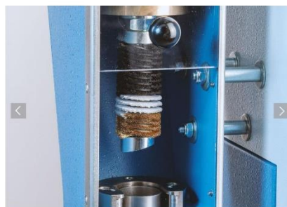
Manual cleaning device for steel rings 40 mm
